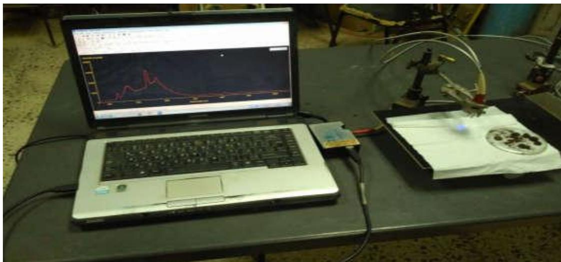
Fig (2.2) the bones samples using USB2000 device to take the energy gap readings
